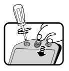
Install 2 new 'AAA' (AM-4/LR03) batteries following the diagram inside the battery box. (The use of new alkaline batteries is recommended for maximum performance.)
